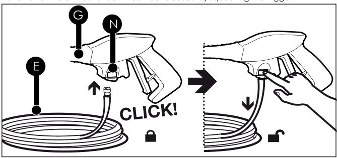
⚠ Make sure the high pressure hose is connected securely to avoid leaks.
